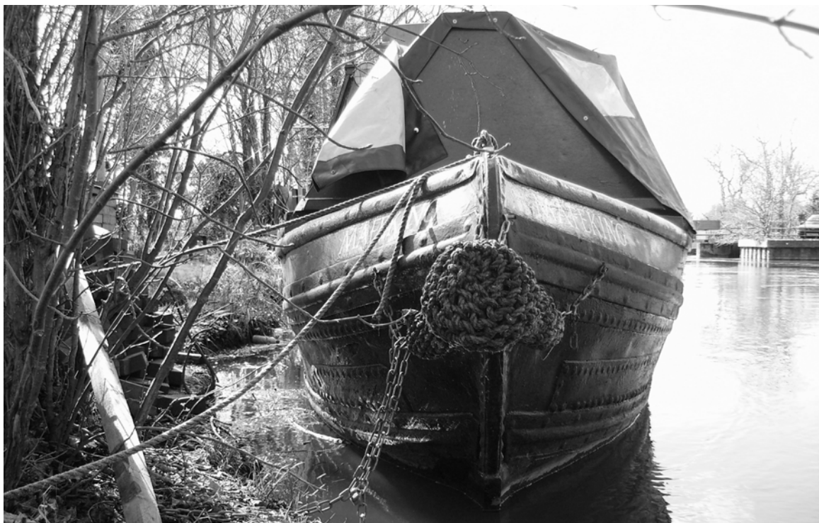
63. Mafeking's distinctive riveted fore-end.
