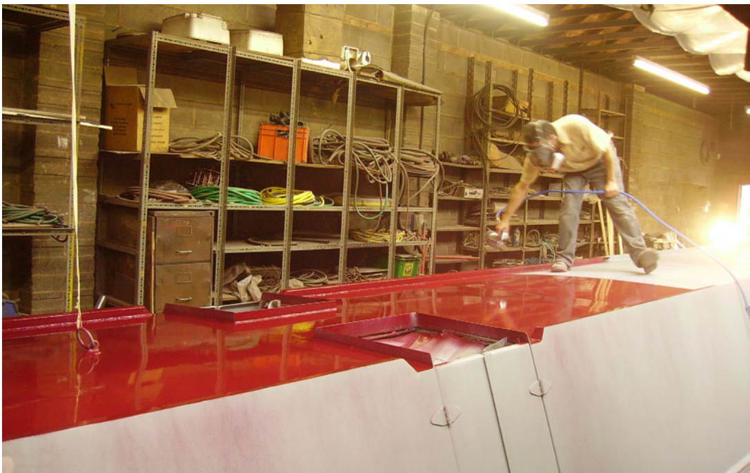
68. Top Right: New steel plates encapsulate the old topsides
